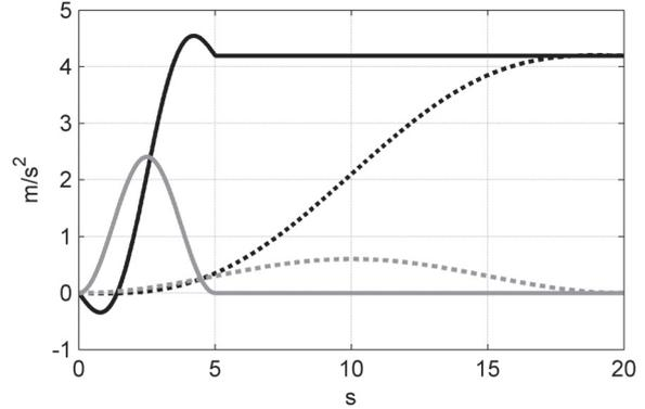
Fig. 3. Forward ( $a_x$ , black lines) and lateral ( $a_y$ , Coriolis, grey lines) accelerations for the two motion profiles used in this experiment: fast ( $T = 5$  s, solid lines), slow ( $T = 20$  s, dotted lines).
